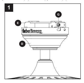
2. Secure the canopy (D) with the mounting bracket screws (Q) previously removed (Step 4, page 8). Tighten all mounting bracket screws (Q) securely.
