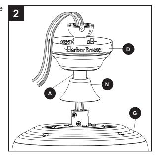
3. Slide the downrod (A) into the yoke of the motor assembly (G), align the holes, then re-install the downrod pin (B) and downrod clip (C). Secure with set screws (S).
