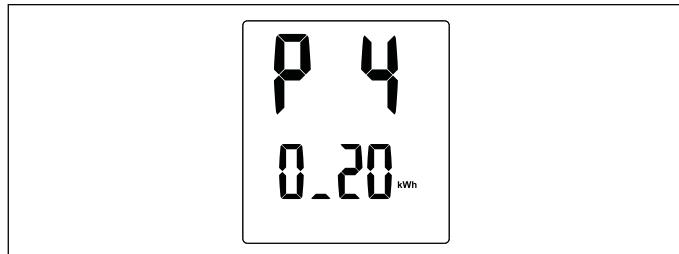
The secondary display will be flashing to indicate that the value can be changed by rotating the control knob. Consult your electricity bill to determine the cost of electricity per kWh.
