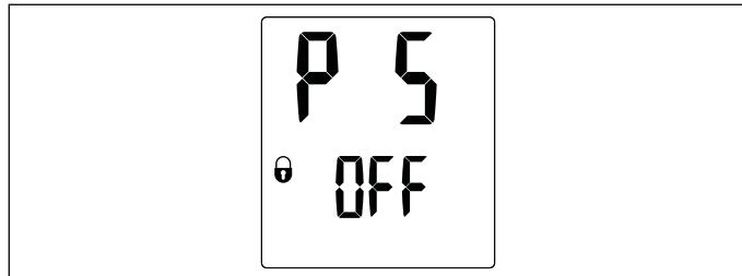
If the display-lock parameter is set to "On" and the user either holds the Information button for 5 seconds or lets the display time out for 15 seconds, the display-lock will become active.
