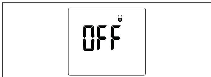
If the display-lock parameter is set to "On" and the user either holds the  $T_{max}$  button for 5 seconds or lets the display time out for 15 seconds, the display-lock will become active.
