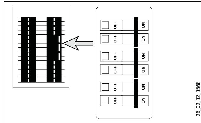
**Tempra 29 or 36 Trend / Plus** These units require three independent circuits. Use three supply cables protected by three separate double pole breakers.
