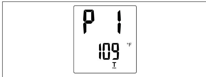
At the T<sub>max</sub> setting menu, the temperature value will flash, indicating that the value can be changed by rotating the control knob. The T<sub>max</sub> value can be increased by turning the control knob clockwise, and decreased by turning it counter-clockwise. The T<sub>max</sub> value can be deactivated by turning the control knob counter-clockwise, past the 68 °F (20 °C) setting. The display will read "Off" if T<sub>max</sub> is inactive.
