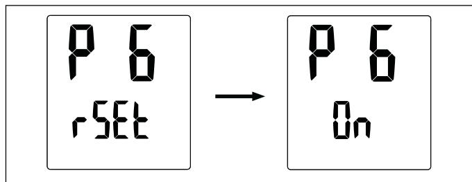
The display will be flashing to indicate that the value can be changed by rotating the control knob. When the value is set to "On", the reset must be confirmed by holding both Button 1 and Button 2 simultaneously for 5 seconds.
