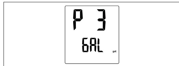
The current volume unit will be displayed and the value will be flashing to indicate that it can be changed. Rotate the control knob to change the value between gallons per minute and liters per minute.
