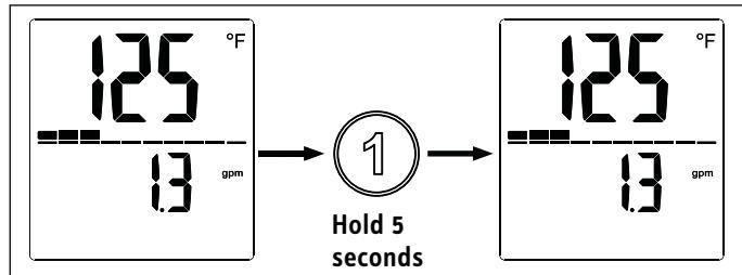
To change the value of either preset 1 or preset 2, first rotate the control knob to the temperature that you want to set the preset value. Then hold the preset button for 5 seconds. The display will flash to indicate that the preset has been changed successfully.
