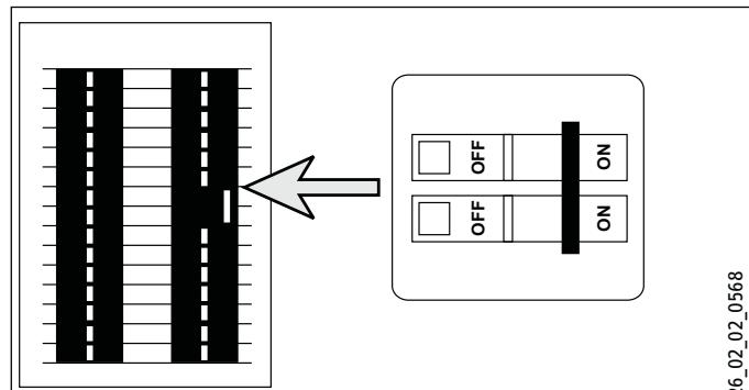
**Tempra 12 Trend / Plus:** These units can be connected to a single circuit. Use a supply cable protected by a double pole breaker.
