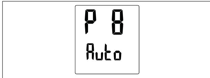
The entire display and backlight will be flashing to indicate that the value can be changed by rotating the control knob. When the value is set to "On", the backlight will always be on. When the value is set to "Auto", it will automatically deactivate after 15 seconds of inactivity.
