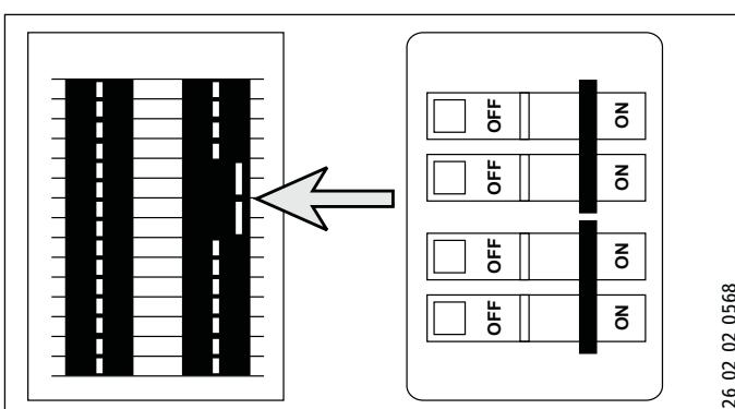
**Tempra 15, 20 or 24 Trend / Plus:** These units require two independent circuits. Use two supply cables protected by two separate double pole breakers.
