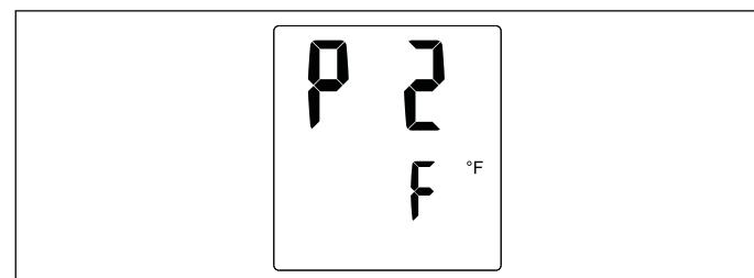
The current unit will be shown and the secondary display value will be flashing to indicate that the value can be changed. Rotate the control knob to change the value between Fahrenheit and Celsius.
