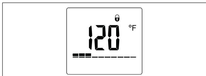
With the display-lock active, a lock will appear on the base display, and no parameters can be changed. In order to disable the lock, hold the  $T_{max}$  button for 12 seconds. The lock will then disappear from the display and all parameters can be changed again.
