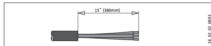
The wire must be fed through the knock-outs located between the hot and cold water connections (See 9.1, "Circuit layout", pg. 12). The "live" wires must be connected to the slots on the terminal block marked L1 and L2. The ground wire must be connected to slot marked with the ground symbol (See 13.3, "Wiring diagrams", pg. 18).
