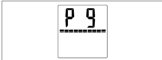
The power capacity status bar indicates the brightness setting. A full capacity bar indicates that the brightness is at the high setting. A half-full capacity bar indicates that the brightness is at the low setting.
