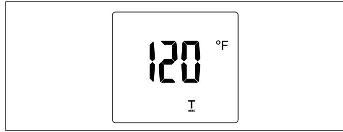
At the  $T_{\max}$  setting menu, the display will flash, indicating that the value can be changed by rotating the control knob. The  $T_{\max}$  value can be increased by turning the control knob clockwise, and decreased by turning it counter-clockwise. The  $T_{\max}$  value can be deactivated by turning the control knob counter-clockwise, past the 68 °F (20 °C) setting. The display will read "Off" if  $T_{\max}$  is inactive.
