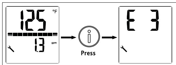
While the wrench is showing, press the Information button to advance the display to the error display page. Consult section "Tempra Plus error code reporting", pg. 14 for information on how to interpret the reported error code.
