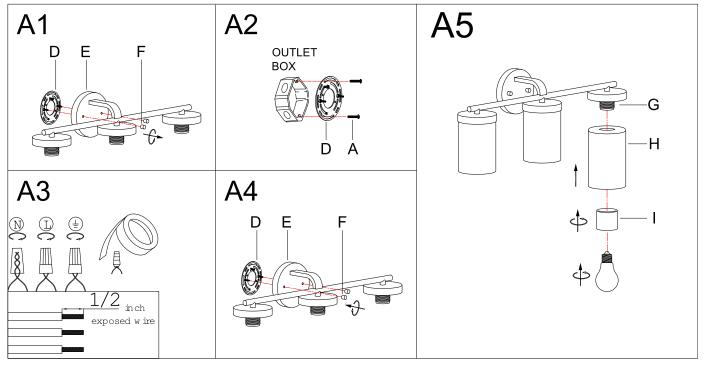
Step A1 » Unscrew knob nuts (F) from back plate (E), then set them aside for later installation.
