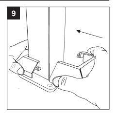
Bring in the second post base piece and rotate it to lock the two pieces together. This will conceal the post flange for a finished look.
