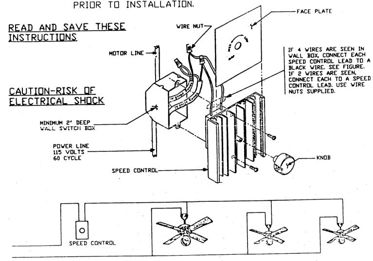
USE OF A LIGHT KIT WITH ANY CEILING FAN DECREASES THE MAXIMUM NUMBER OF FANS THAT MAY BE SAFELY USED WITH THIS CONTROL. ADD UP THE TOTAL WATTAGE OF LIGHT BULBS BEING USED, DIVIDE BY 120, AND SUBTRACT THIS RESULTANT LINE CURRENT FROM 15 AMPS. WHATEVER IS LEFT IS THE MAXIMUM CURRENT THAT THE TOTAL NUMBER OF CEILING FANS CAN DRAW. FOR SAFETY, CONSIDER THAT EACH 52" FAN MOTOR DRAWS 1.0 AMPS. AND EACH 42" FAN DRAWS 0.6 AMPS OF LINE CURRENT.
