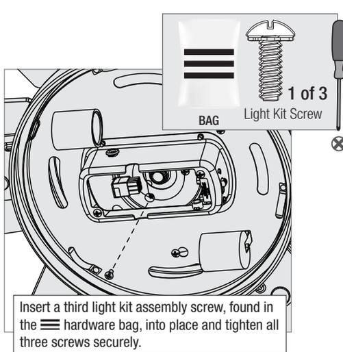
Insert a third light kit assembly screw, found in the
