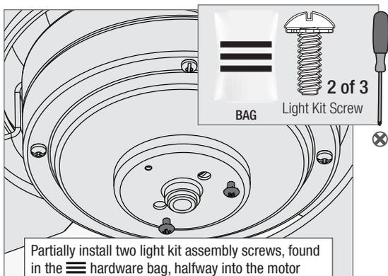
Partially install two light kit assembly screws, found in the
