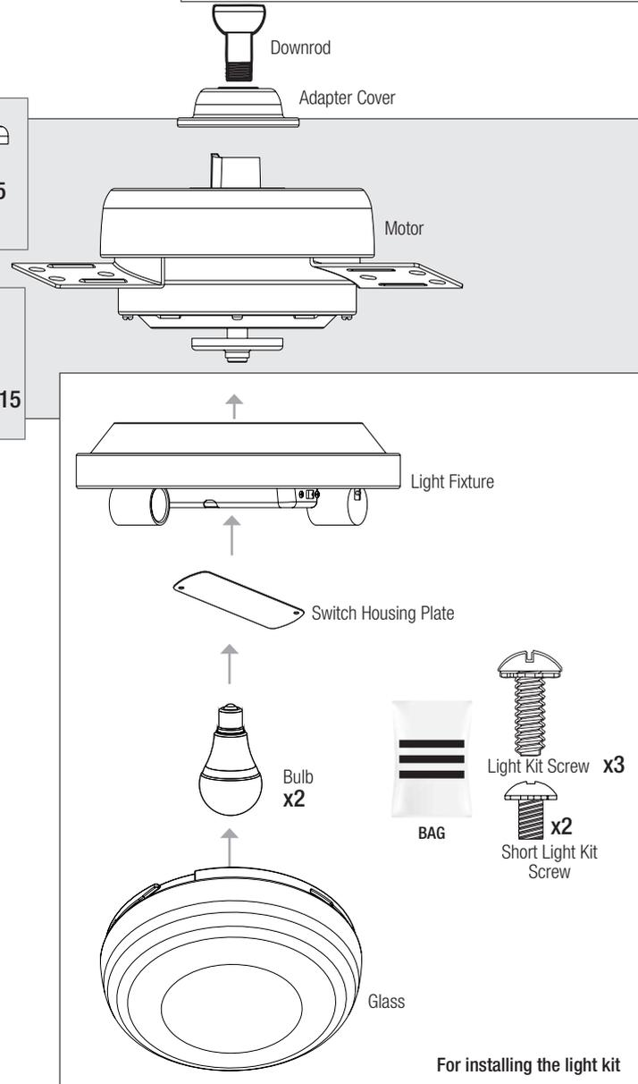
For installing the light kit
