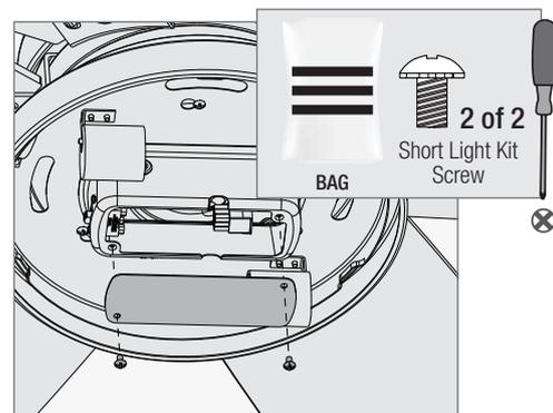
Carefully push all switch housing components into the switch housing, then install the switch housing plate using two light kit assembly screws, found in the
