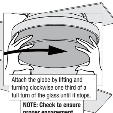
Attach the globe by lifting and turning clockwise one third of a full turn of the glass until it stops.
