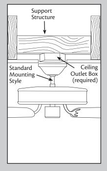
Use **Standard Mounting** to hang the fan from a flat ceiling.
