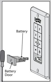
To change the battery, push on the battery door to eject it.
