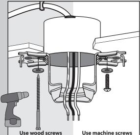
(included) when securing to support structure with approved electrical outlet box. Drill 9/64" pilot holes in support structure to aid in securing ceiling bracket with hardware found in the ★ hardware bag.
