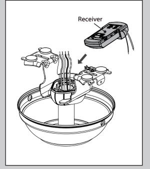
Place the receiver on top of the downrod assembly as shown.
