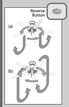
The reverse button on the wall control changes the air flow direction. In warm weather, use (a) downward air flow pattern. In cold weather, use (b) upward air flow pattern.
