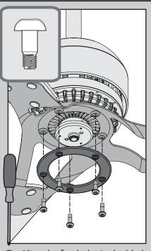
Align the five holes in the blade iron assembly and the decorative ring with the five holes in the bottom of the motor and partially install the five blade iron screws, found in the X hardware bag. Once all five screws are partially installed, tighten them securely.
