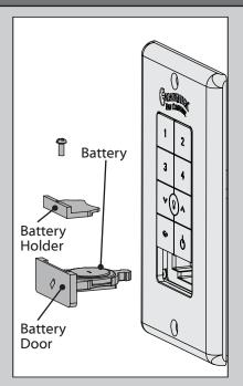
Before operating the wall control, press on the battery door to eject it.
