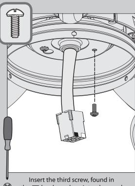
the hardware bag, into place and then tighten all three screws.
