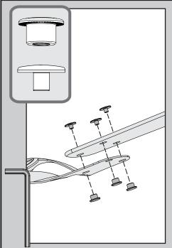
Using the provided Allen wrench, attach each blade to the blade iron assembly using three barrel nuts, found in the ■ hardware bag, and three decorative screws, found in the ▲ hardware bag.
