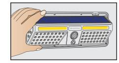
Press the unit firmly onto the surface for a few seconds.
