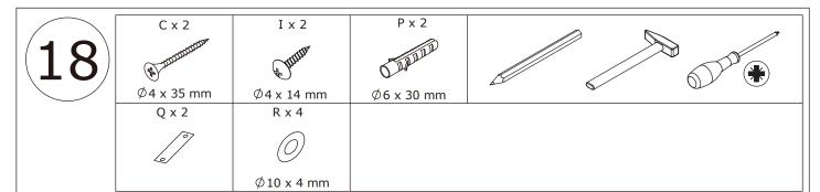
For extra stability, it is recommended that you fix your drawer to the wall using the additional hardwares (C, T, R,P and Q), as shown.
