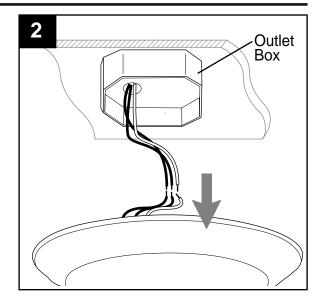
Attach mounting strap (C) to outlet box (not included) using existing washers and outlet box screws or the machine screws (BB). NOTE: If the outlet box screws required for your outlet box are of a different size than the machine screws (BB), consult a licensed electrician before proceeding.
