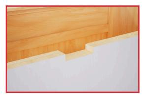
1. Mark 2"-4" from the outer edge of the the cabinet for your first notch to be cut. Then set marks for the remaining brackets every 16"-20" apart. With your brackets properly spaced, rout or chisel a 2.5" wide by 0.5" deep notch for each bracket.
