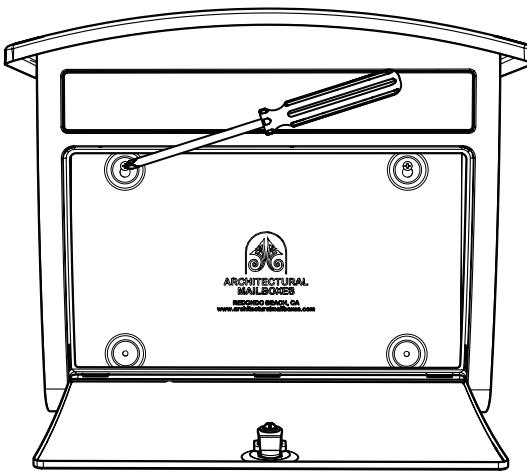
**5** While the mailbox is hanging on the top screws, insert the remaining two screws into the bottom holes and secure with a screwdriver.
