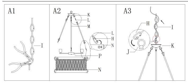
Step A1: By measuring, determine the correct number of links needed for proper hanging height. Using the chain pliers, disconnect and discard the remaining chain.
