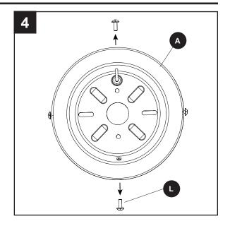
5. Feed the supply wires from the outlet box through the center hole in the mounting bracket (A). Then, secure the mounting bracket (A) to the outlet box (not included) using screws and washers provided with the outlet box.
