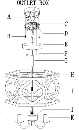
2. Unscrew knob nuts (F) from canopy (E), then gently remove mounting plate (C) from canopy (E) and set them aside for later installation.
