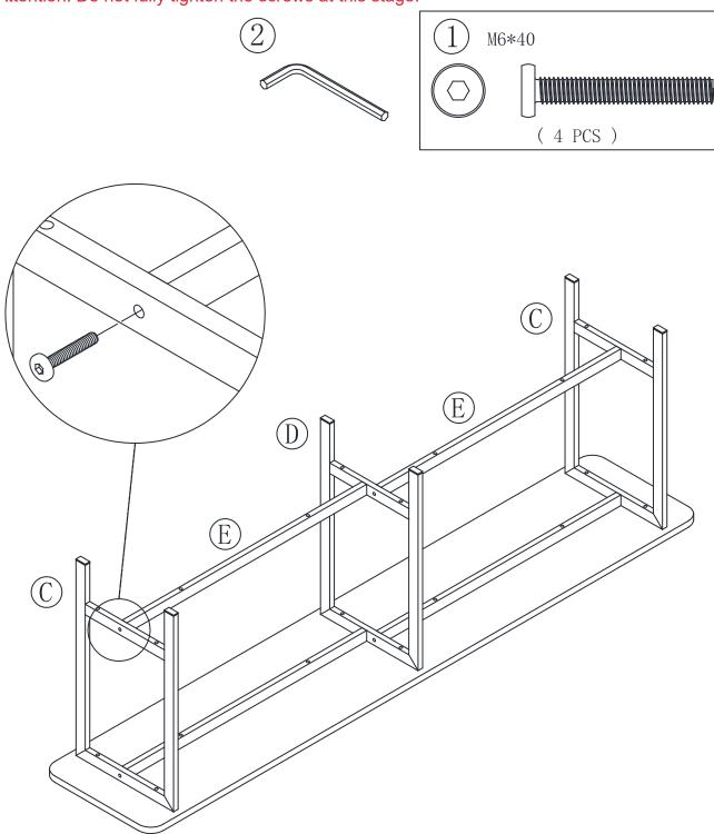
Now you can fully tighten all screws from Step 1 to Step 4
