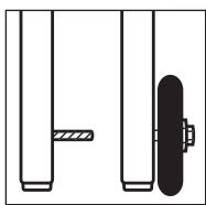
3 Flip up tray to horizontal, adjust horizontal height until it is level with the height of your table saw
