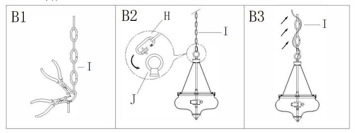
Step B1: By measuring, determine the correct number of links needed for proper hanging height. Using the chain pliers, disconnect and discard the remaining chain.
