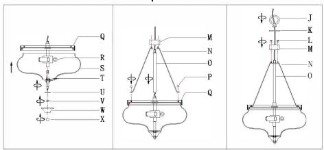
Step A1: Screw the screwed pipe (T) to the joint of the flat iron ring (Q), fix the glass shade (S) and the plastic washers (U) on the screwed pipe (T) with the hex nut (V). Cover the glass shade (S) with a flat cover (W), then secure the lock with a ball nut (X). Step A2: Fix the arms (N) to the flat iron ring (Q) with nut (P). Screw the tube (O) to the flat iron ring (Q).
