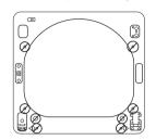
e. Remove the three screws on the hinge at the bottom left. Remove the hinge and reinstall it on the right side. The top screw will occupy the hole where you removed the screw behind the hinge bracket in step d.
