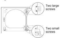
b. Lift the door slightly to disengage the hinge support and remove the door from the cabinet. Set the door aside face down on a protected work surface.
