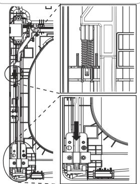
Reinstall the side interlock button. 12 Install the side interlock button on the opposite side from which it was removed.
