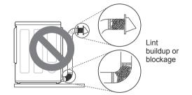
Make sure the ductwork is not crushed or restricted.
