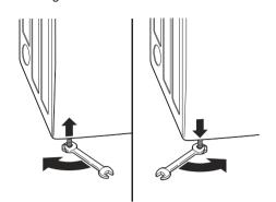
If you are installing the dryer on the optional pedestal, you must use the leveling feet on the pedestal to level the dryer. The dryer leveling feet should be fully retracted.
