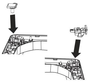
f. Insert and tighten the screw connecting the upper hinge assembly to the top lock rod, removed in step a.
