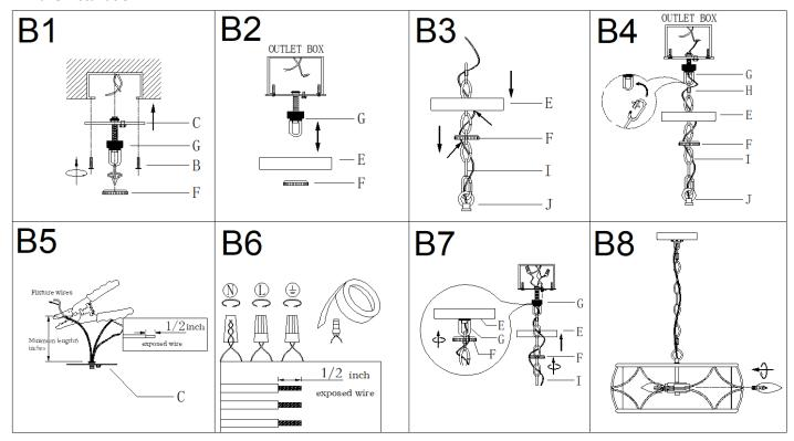
Step B1: Remove the collar ring (F) from collar loop (G). Attach the single bar (C) to outlet box with mounting screws (B). NOTE: the side of single bar marked "GND" must face out.
