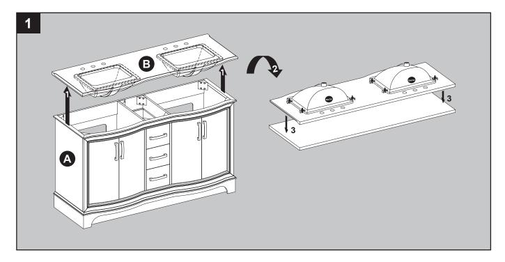
**Note:** Clean area where the vanity (A) will be permanently located prior to beginning installation, ensuring the vanity (A) will not interfere with any water supply and drain lines once mounted.
