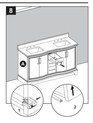
9. To reinstall drawer(s) into vanity (A), fully extend metal glide tracks. Gently lower and slide drawer box into rear glide catch. Next, lower drawer box down to completely rest on extended glides. Then, push plastic levers to lock the drawer box in place. Repeat for remaining drawers.
