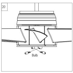
Install 2 G9 35W bulb. Bulb included. **Warning**: Over lamping the fan will result in the fan lights shutting down until the proper wattage of bulbs are installed. Reset the lights by turning off, replace bulbs with the correct wattage bulbs, turn the power on.
