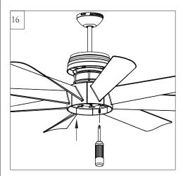
Lift blade assembly up. Aligning the holes on the coupler and the screw holes on motor and then install it onto motor using the screws provided. Tighten screws securely.
