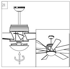
Attach glass to light pan by locating dimples in light pan with grooves on the glass and twist clockwise until tight.
