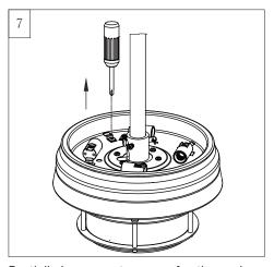
Partially loosen set screws for the spring clips
