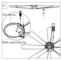
Flip the blade assembly over and install blade supporting ring onto the blades with screws provided.
