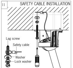
For Canadian installation and for USA fan and light kit combinations over 35 lbs, in both flush and downrod mode the safety cable must be installed into the house structure beams using 3" lag screws, washers and lock washers provided. Make sure that when the safety cable is fully extended the lead wires are longer than the cable and no stress is placed on the lead wires.
