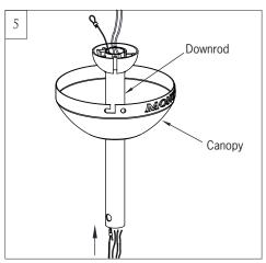
Place downrod over canopy. Thread lead wires and safety cable from motor assembly through downrod.
