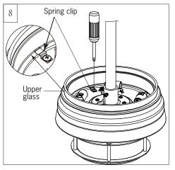
Place upper glass on top of fan. Adjust the spring clips to hold the glass in place. Tighten all set screws securely.
