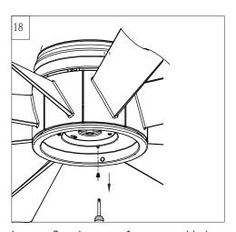
Loosen 2 and remove 1 preassembled screw from the light pan. Save screw for later use.
