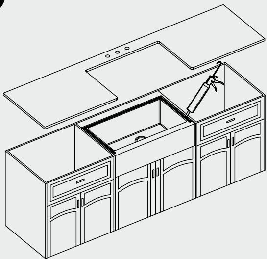
Use a bead of silicone (or preferred adhesive) around the rim of the sink. Check the alignment of the sink to the cutout in the countertop. Place the countertop cutout hole over the sink and press firmly. Remove excess silicone with a wet rag.
