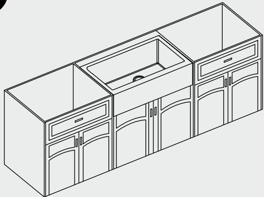
Place the sink in the opening. The weight of sink should be sustained by the built supports. Make sure sink is level from front to back and side to side. Ensure the top surface of the sink rim is flush with the tops of the cabinet walls. Position the sink so that the sides of the apron are recessed into the face frame of the cabinet by an appropriate amount depending on personal preference.
