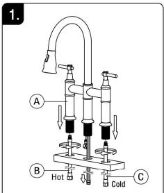
Connect the hot and cold Supply Hoses (B&C) to the main Body(A), then put the fauce into the mounting hole.
