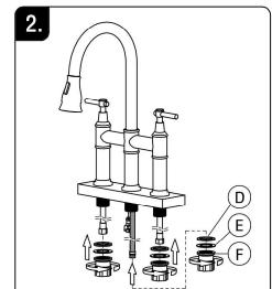
Use Nuts(F) to fix the faucet. Rubber Washer (D) and Metal Washer (E) are required between the Nuts and the fixing plate.
