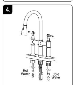
Last but not least, connect the Supply Hoses(B&C) to the water supply valve. Faucet installation completed.
