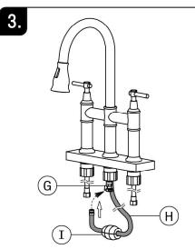
Conect the Spray Hose(H) to fast-inserting Joint (G). Then install the Weight (I) to the proper place on the Spray Hose.
