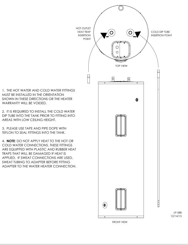
Figure 3 - Installing Cold Inlet and Hot Outlet Fittings
