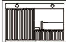
1.Remove the grease filter one by one by pushing down each latch.This will disengage the filter from the hood.Tilt the filter downward and remove.
