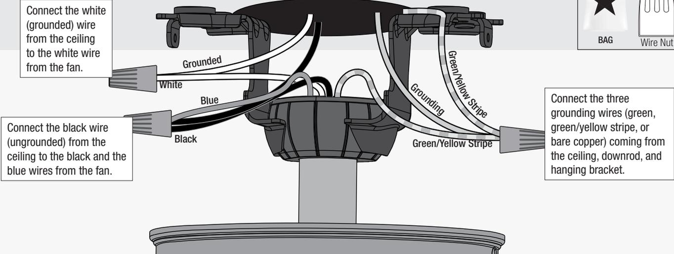
**⚠ WARNING** The ceiling fan must be grounded. If the ground wire for the installation site is not present, immediately **STOP** installation and consult a qualified electrician.
