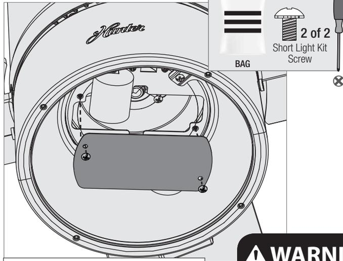
Carefully push all switch housing components into the switch housing, then install the switch housing plate using two short light kit assembly screws, found in the hardware bag.
