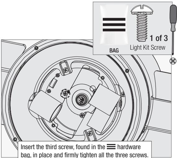
Insert the third screw, found in the hardware bag, in place and firmly tighten all the three screws.
