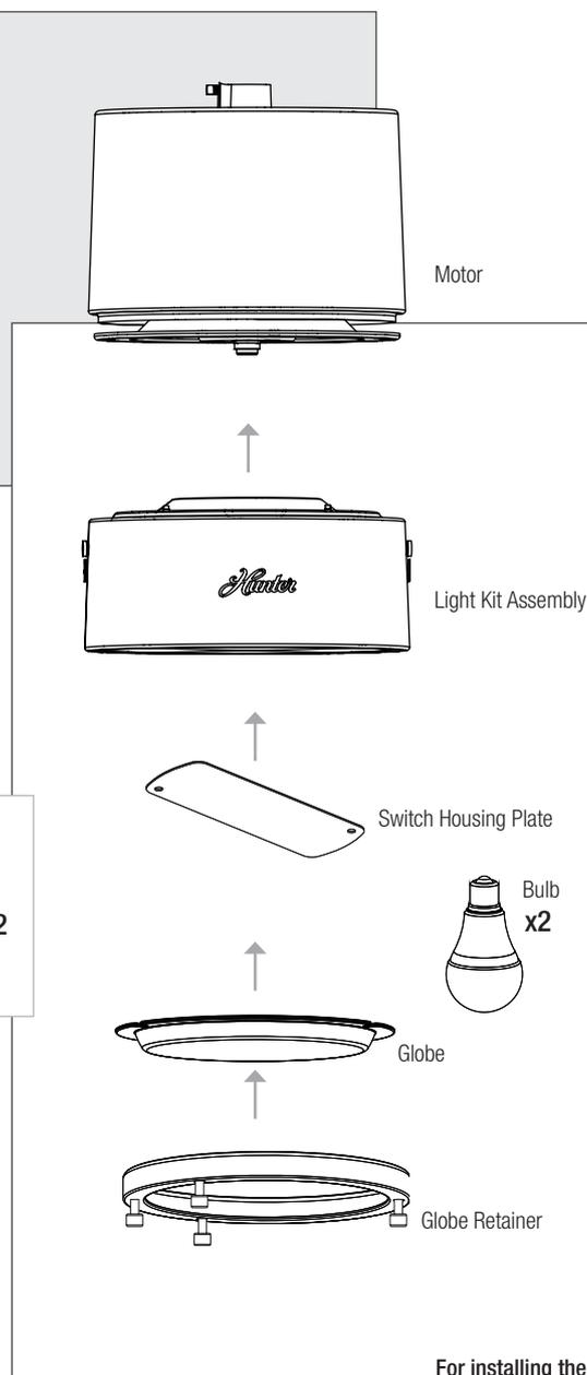
For installing the light fixture
