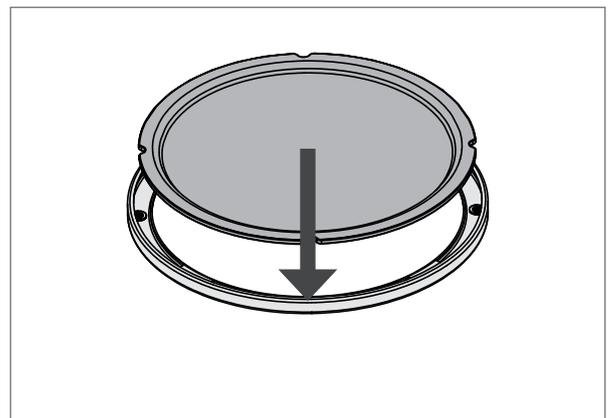
Align the globe indentations with the globe retainer screw holes and carefully lower the globe into the globe retainer until it rests in place.
