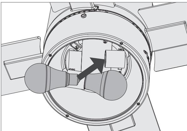
Install a bulb into each of the sockets. When necessary, replace with bulbs of the same wattage.
