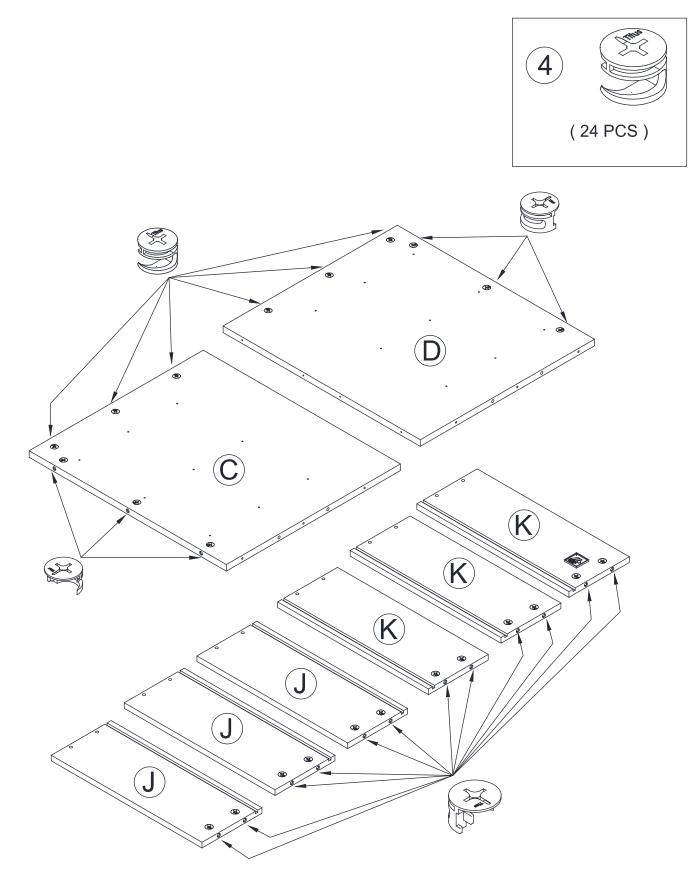
◆ Fasten the FRONT MOLDING (E) to the LEFT END (C) and the RIGHT END (D) by fasten the HIDDEN CAM (4).
