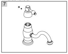
Turn off water and relieve pressure before working on your faucet! Unscrew Handle Assembly, then pull out handle assembly from valve stem with force.
