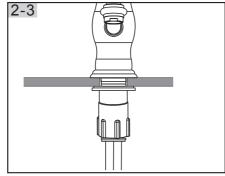
If necessary, tighten mounting nut using a Adjustable wrench until the faucet is firmly connected to the Wash Basin.
