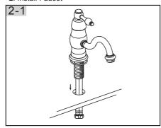
Make sure the Rubber Washer is placed onto the bottom of Base Ring. With the Handle and spout facing forward, install faucet through the hole in the sink.
