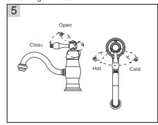
Lift the handle up, the cartridge will be activated allowing water to flow. The water flow will increase by continuing to rotate handle. By rotating the handle to the right, the water temperature will decrease to cold flow only. By rotating Handle to the left, the water temperature will increase to hot only.
