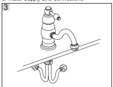
Connect hot and cold water flexible hoses to the Water Supply Valves.
