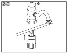
From underside sink, place Plastic Washer and Metal Washer onto screw tube and tighten with Mounting Nut by hand. Before final tightening, make sure Spout and Handle facing forward.
