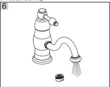
After installation is complete, remove aerator and rotate handle to the close position. Turn Water Supply Valves on, and check all connections for leak. Turn faucet on and allow both hot and cold water to run at least one minute each. Replace Aerator.
