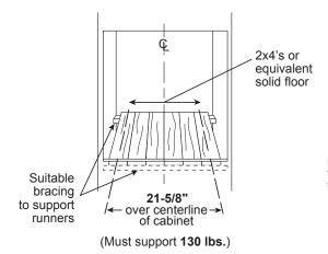
Note: Cabinets installed adjacent 23-1/2" to wall ovens must have an adhesion Cutout depth spec of at least 194° F temperature rating. 25-1/4" 4-3/16" Cutout width 21-1/2" Back of Control Junction box location Conduit 17-1/2" Construct Solid 20-1/8" (48-1/2) Cutout height Bottom MIN. long) 3/8" Plywood Supported by 2 x 4 or 1 x 2 Runners, all four Sides. (Must Support 5" MIN. from 150 lbs.) floor 1" MIN. above toekick Four Sides. 26-3/4" 30"
