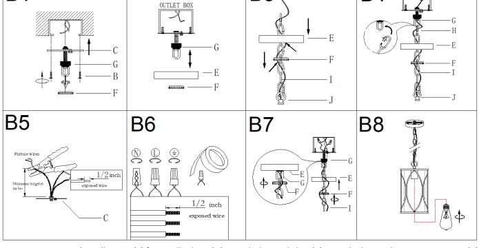
Step B1: Remove the collar ring (F) from collar loop (G). Attach the single bar (C) to outlet box with mounting screws (B). Note: the side of single bar marked "GND" must face out.
