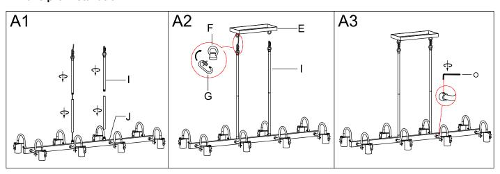
Step A1 » 1) Carefully pass the fixture wires through one side of tubes (I) and loops (F).
