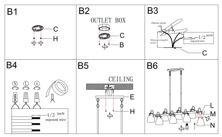
Step B1 » Unscrew ball nuts (H) from mounting plate (C).
