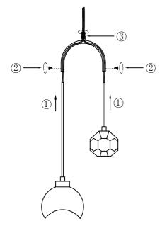
① Two wires are respectively threaded through all curved pipes, and two wire cores with white markings are pulled out from the middle vertex hole, forming one group in parallel and the other group in another
