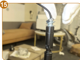
Remove the nut and gasket from the universal joint for later use.
