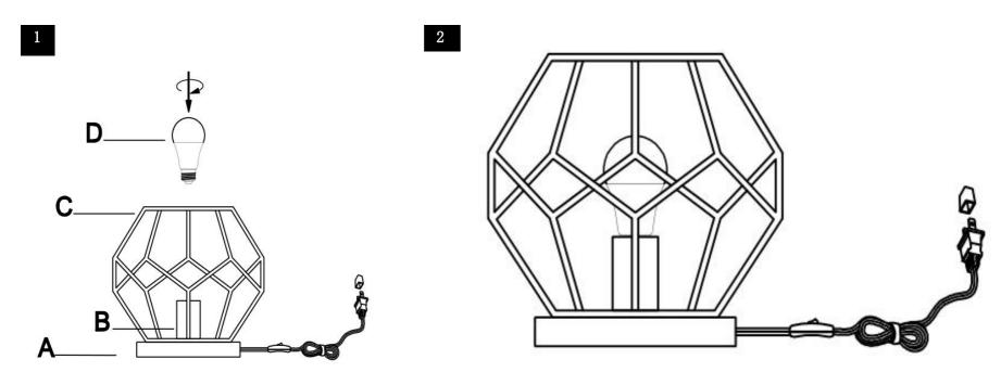
Step 1 Insert the bulb(D) into the socket(C).
