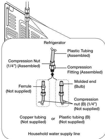
1. Connect the household water line to the assembled compression fitting.
