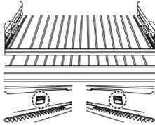
5. Holding the top of the Freezer Drawer, pull it out all the way, and then remove it from the rail system.
