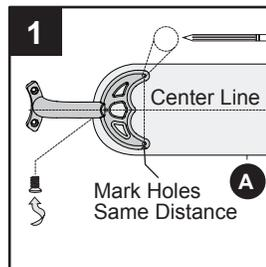
**CAUTION:** It is extremely important that the blade arm screw holes are aligned and centered properly before drilling any holes. Failure to do this may result in unbalanced fan operation or wobble.
