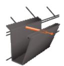
Spike & Ferrule Insert femule into gutter lined up with a rafter, hammer spike through gutter and drip edge into the fascia.
