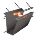
Hidden Hanger Hook the hanger under the front lip of the gutter. Drive a nail or screw through the hole in the hanger into the fasda.
