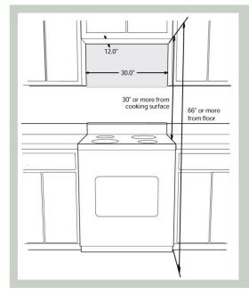
Each Sharp Over the Range microwave oven can be easily adapted for either outside ventilation (vertical or horizontal) or non-vented, ductless recirculation. Make sure the top of oven will be at least 66" from the floor and at least 30" from the cooking surface. A separate 15 amp. or greater electrical receptacle must be located in the cabinet directly above the microwave oven.
