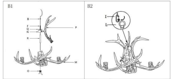
Step B1: Unscrew the ball nuts(N), hex nust(B) from the antler(P). Carefully push the antler to make the threaded nipple through the hole on trim, then secure with hex nuts(B), The sleeve (R) screw into the antler chandelier main body(M), then the cover plate(Q) and the teeth are screwed, through trim(N) into the other end of the sleeve(R), then secure with hex nuts(B). Fix the loop(L) onto the threaded nipple(F).
