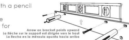
**2** Using a power drill and 9/32" drill bit, drill hole into wall marks. Using a power drill or screwdriver, (for Phillips head screw), drive provided screws into studs (or anchors), securing backplate to wall.
