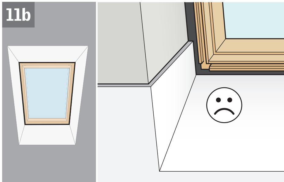
**ENGLISH:** If the drywall is not installed tight into the lining groove, add on-site insulation and trim for finished appearance and to prevent conditions that may contribute to condensation.
