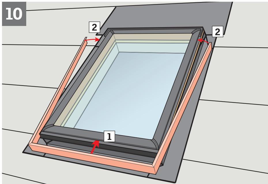
**ENGLISH:** You are now ready to install the flashing. If the flashing is not to be installed immediately, reinstall cladding.
