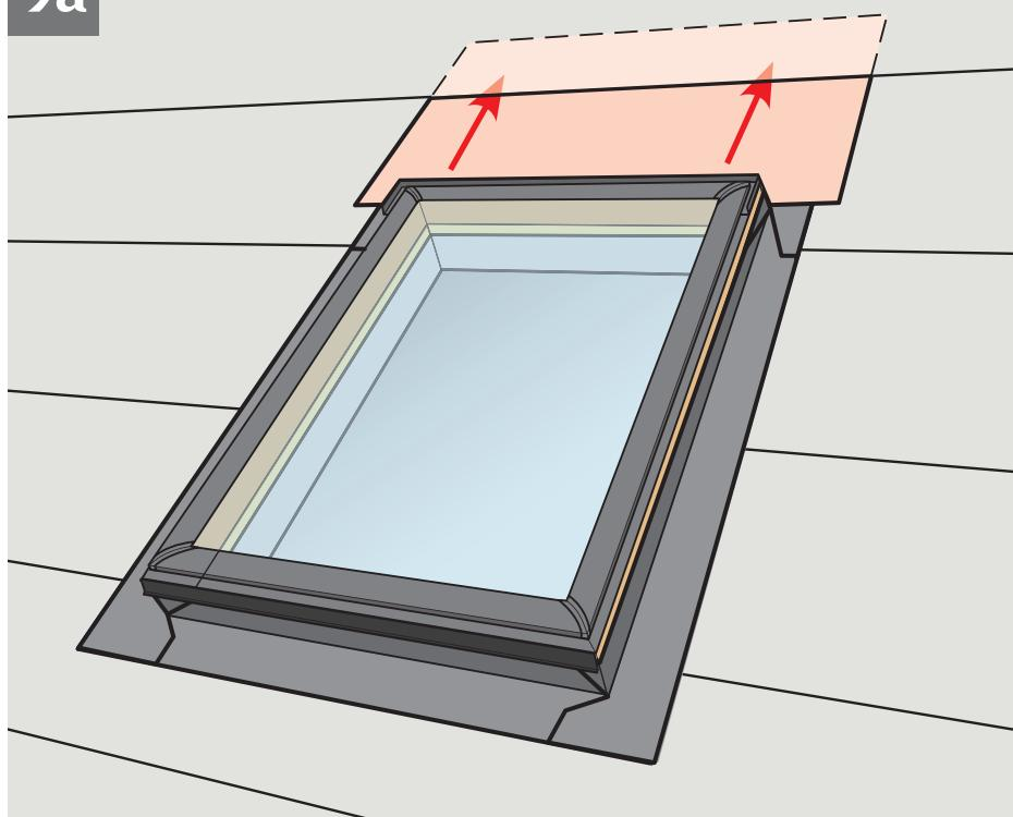
**ENGLISH:** To allow for proper drainage, interweave roofing underlayment as shown in **9a** for new construction applications. For retrofit applications, interweave roofing underlayment as shown in **9b**.
