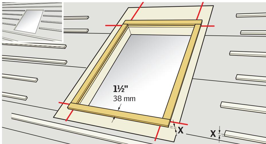
**ENGLISH:** **Rough opening:** Place 1 1/2" (38 mm) wide battens around rough opening. Batten thickness around rough opening should be equal to thickness of battens used for roofing material.
