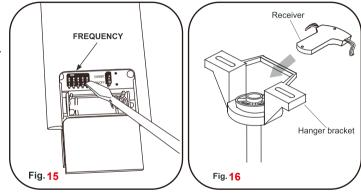
Step 2. Motor to Receiver Electrical Connections:
