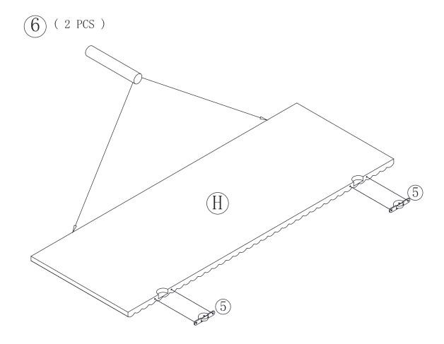
◆ Place the bolts of the DOOR (H) to the groove on the TOP (A).
