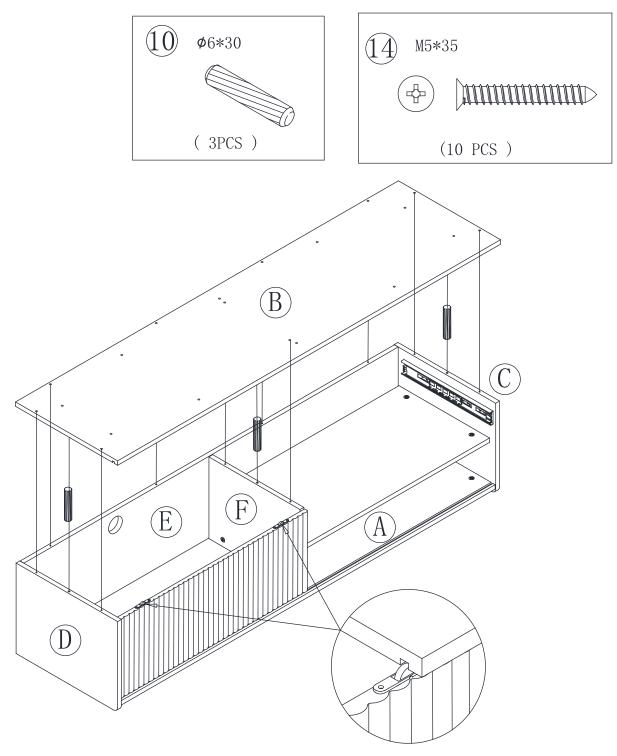
Note: Be sure the LOWER DOOR BRACKETS into the groove on the BOTTOM (B)
