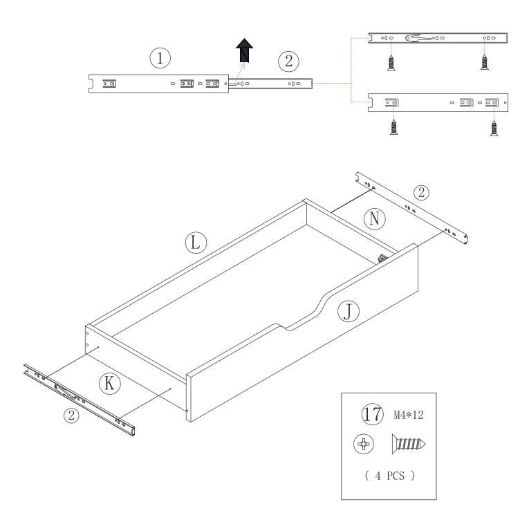
To insert a drawer into your unit, line up the EXTENSION SLIDES on the drawer with the EXTENSION RAILS on the
