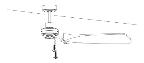
Remove the pre-installed screws.
