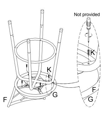
Stand chair up on an even surface and check that it is balanced. If there is a slight wobble, apply downward pressure in the corner where a leg is uneven. Keeping pressure in that corner, tighten all bolts. If balanced, apply downward pressure evenly in the center and tighten all bolts. Do not over-tighten beyond hole depth.
