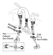
Turn on the water supplies. Check all connections for leaks.
