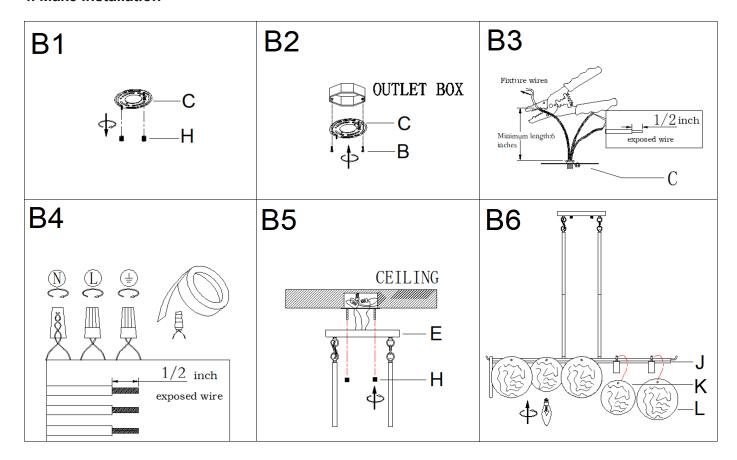
Step B1 » Unscrew knob nuts (H) from mounting plate (C).
