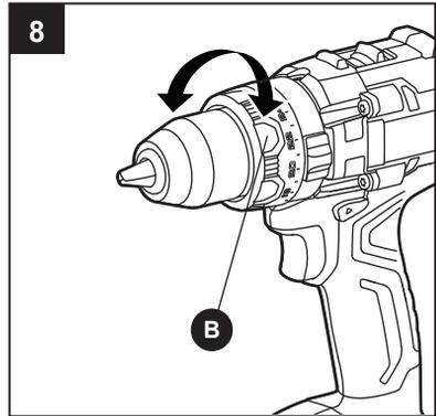
**NOTICE:** Do not change the torque setting when the tool is running.
