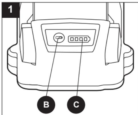
**NOTICE:** The power indicator can be used whether the battery is attached or removed from tool.
