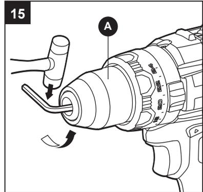
**NOTICE:** The chuck screw has left-handed threads. Attach a new chuck to the spindle and tighten the chuck screw.
