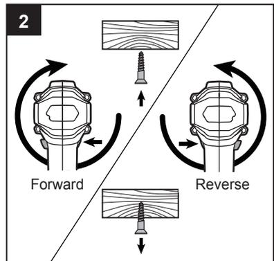
**NOTICE:** To prevent gear damage, always allow the hammer drill to come to a complete stop before changing the direction of rotation.
