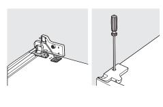
15. Replace upper door. Place door on middle hinge and align with cabinet ensuring that the door gasket seals tightly with cabinet. Secure the top hinge tightly to the cabinet.
