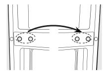
9. Remove the adjustable feet from both sides. (See Figure A.) Remove the bottom hinge. (See Figure B.)
