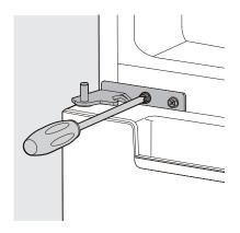
16. Connect door switch terminals to top hinge cover. Screw top hinge cover in place.
