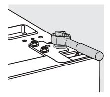
4. Remove pin with adjustable wrench. Flip hinge bracket over, attach pin to opposite side of bracket.
